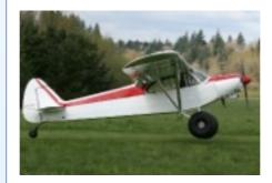
Piper Super Cub N 7878D Fuel Capacity: 67 US gallons Fuel flow: 8 US gallons per hour True air speed: 80 knots Endurance: 8.3 hours - 664 Nm
